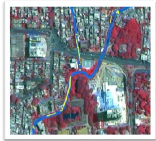
Overlap of sewer line (yellow colour) and drain (blue colour)
