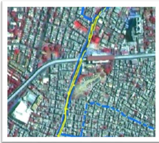
Overlap of sewer line (yellow colour) and drain (blue colour)
