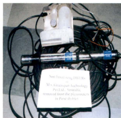
Non functional Digital Water Level Recorder declared irreparable
