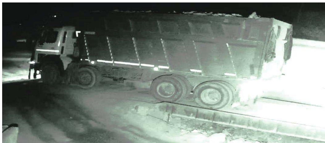
Figure 22: Images in figure 21 and close up image of vehicle in figure 22 showed that minerals were loaded upto the top of the vehicle. Further, loading of 14.5 MT of mineral was not possible.
