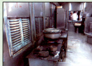
Fig. 1: Use of open flame gas burner in Train No. 12955 Mumbai Central-Jaipur Superfast Express (07.10.2016)
