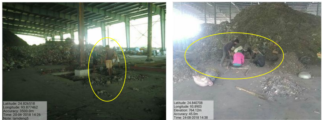
Workers without any masks, gloves, boots, jackets, etc. at Lamdeng Plant (20 June 2018 and 24 August 2018)
