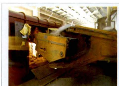
Mechanised loading of cement being done in a wagon in South East Central Railway
