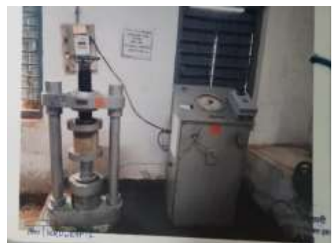
2. Compressive strength Testing machine Dated: 04.10.2021(Janjgir lab)
