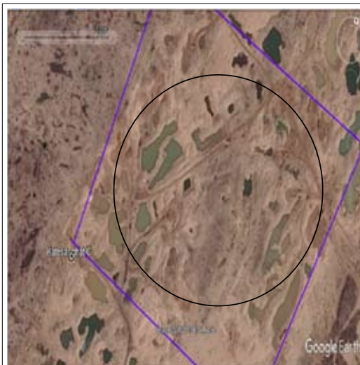
Figure 71: Satellite image of Kateshar sand ghat on May 2016 where sand extraction can be seen in circle.
