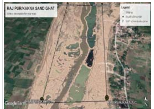
Figure 31: Rajipur/Kakna sand ghat area allowed for mining was in middle of the river.
