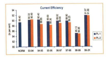
Note: Current efficiency is expressed as percentage of actual aluminium produced (per day/Kg.) to the theoretical maximum production per unit of current flow (ampere).
