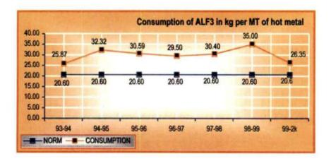
Due to consumption of aluminium fluoride in excess of norm the Company had to incur an additional expenditure of Rs.45.11 crore during the seven years ended March 2000 (Annexure-V).
