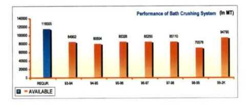
The maximum bath crushing in the last seven years was 94790 MT in 1999-2000. Thus, shortfall in supply of crushed bath led to inadequate covering of anodes resulting in pot instability, increased pot voltage, air burning of anode, pin exposure and fallen anodes.
