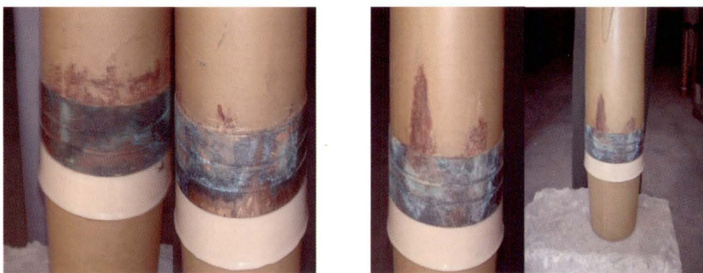
Rejected 155 mm Ammunition due to corrosion
