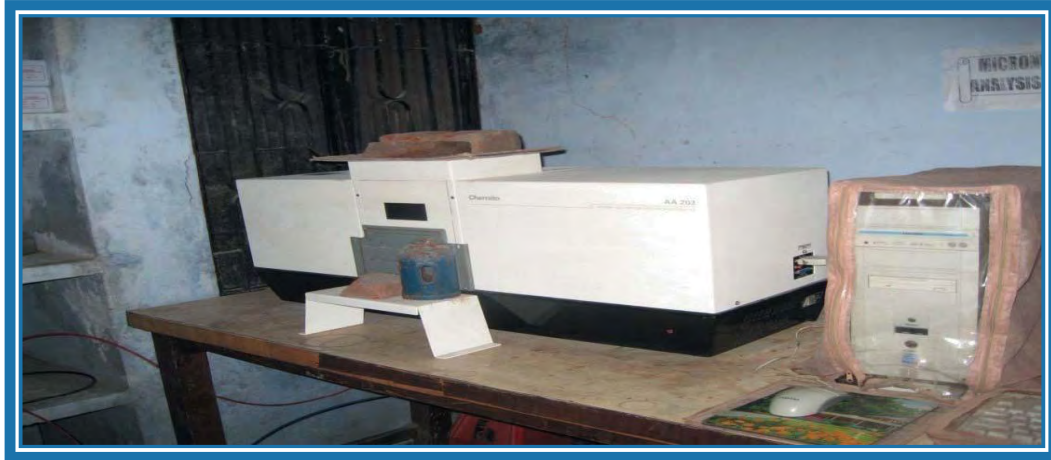
Bricks lying atop non functional Atomic Absorption Spectrophotometer at Srinagar, Pauri laboratory
