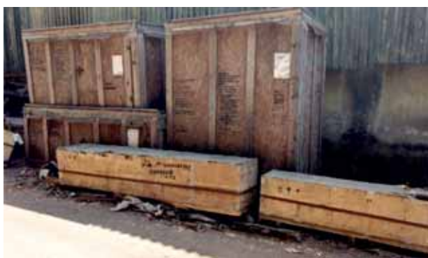
Items marked for storage in covered sheds lying in open
