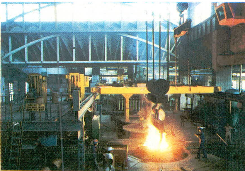
Molten metal in ladle lowering to pouring p
