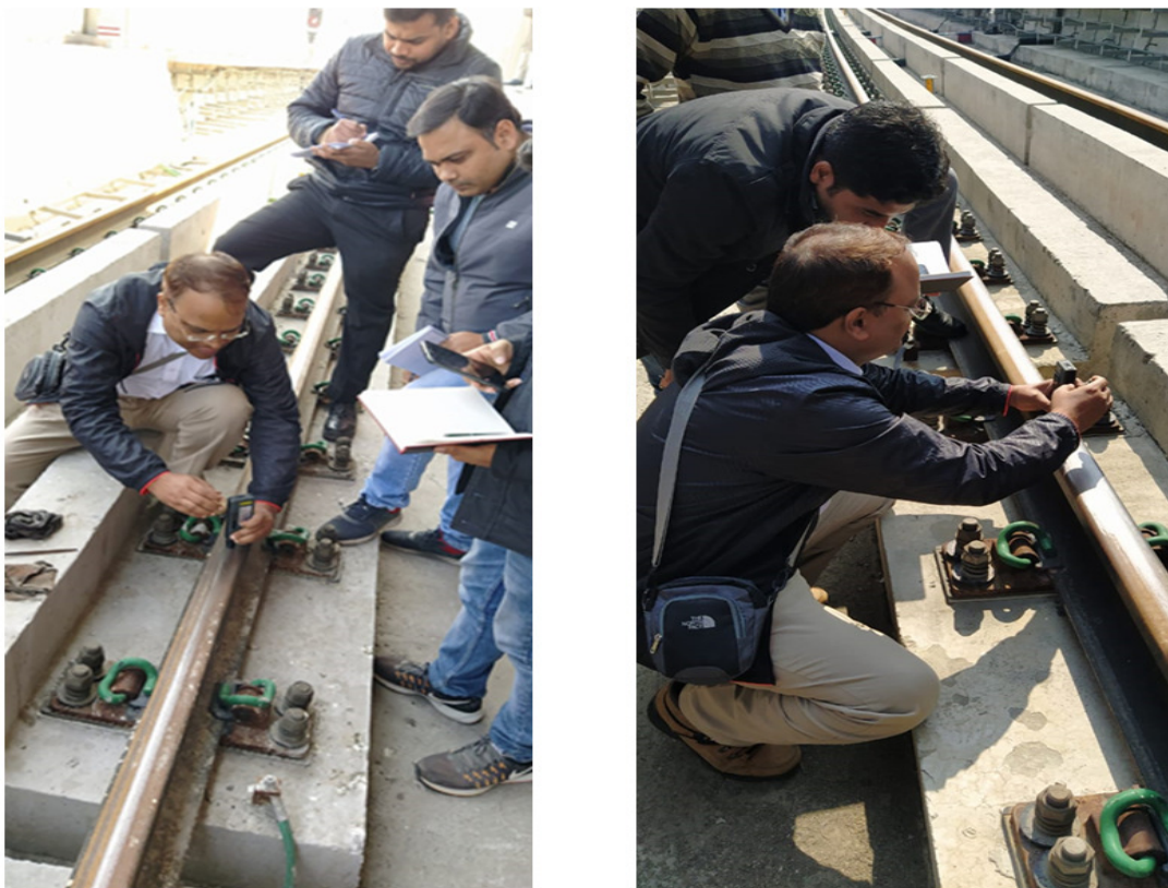
Figure 2.2 Measuring of rail surface hardness of Line-7 (IP extension metro station on 31 January 2020)
