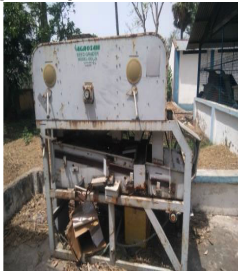
Figure 2.1.8 : Damaged Seed grader lying in open threshing floor in SARF Kandi
