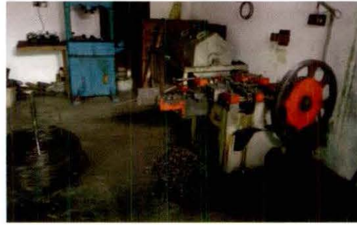
Picture 6.3: Non-fencing/guarding of moving parts of nail cutting machine – Kerala Wires and Nails, Payyoli, Kozhikode (21 May 2017)
