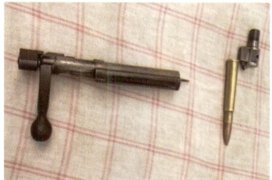
Glimpse of a defective pin and ejector
