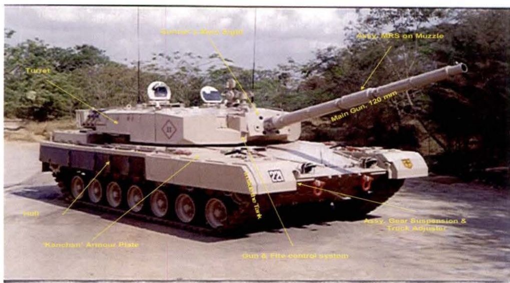
MBT – Arjun and its major assemblies Table-46: Delays in supply of major assemblies
