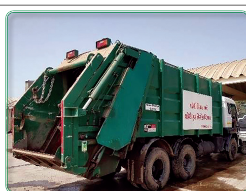
Picture 4: RCVs supplied to 25 NPs without footsteps and hand bars. Photograph of Bharuch NP is illustrated here (18.05.2018)
