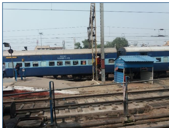
Fig.4.1 Train no. 12948 (Azimabad Express) having 23 coaches stopped at Platform no.3 (handling capacity of 15 coaches) at Kanpur Central Junction on 26.10.2017
