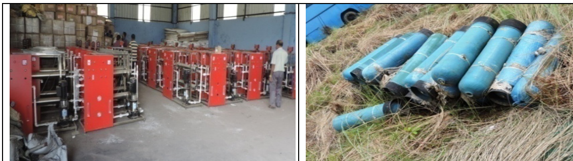
Solar Operated Reverse Osmosis Plants lying uninstalled (27 July 2017)
